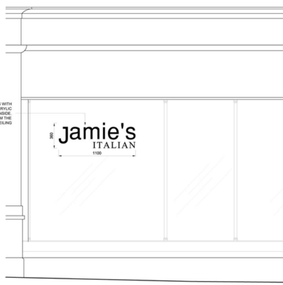
02 HANGING SIGN & WINDOW SIGN - EAST ELEVATION 1:20 @ A1
