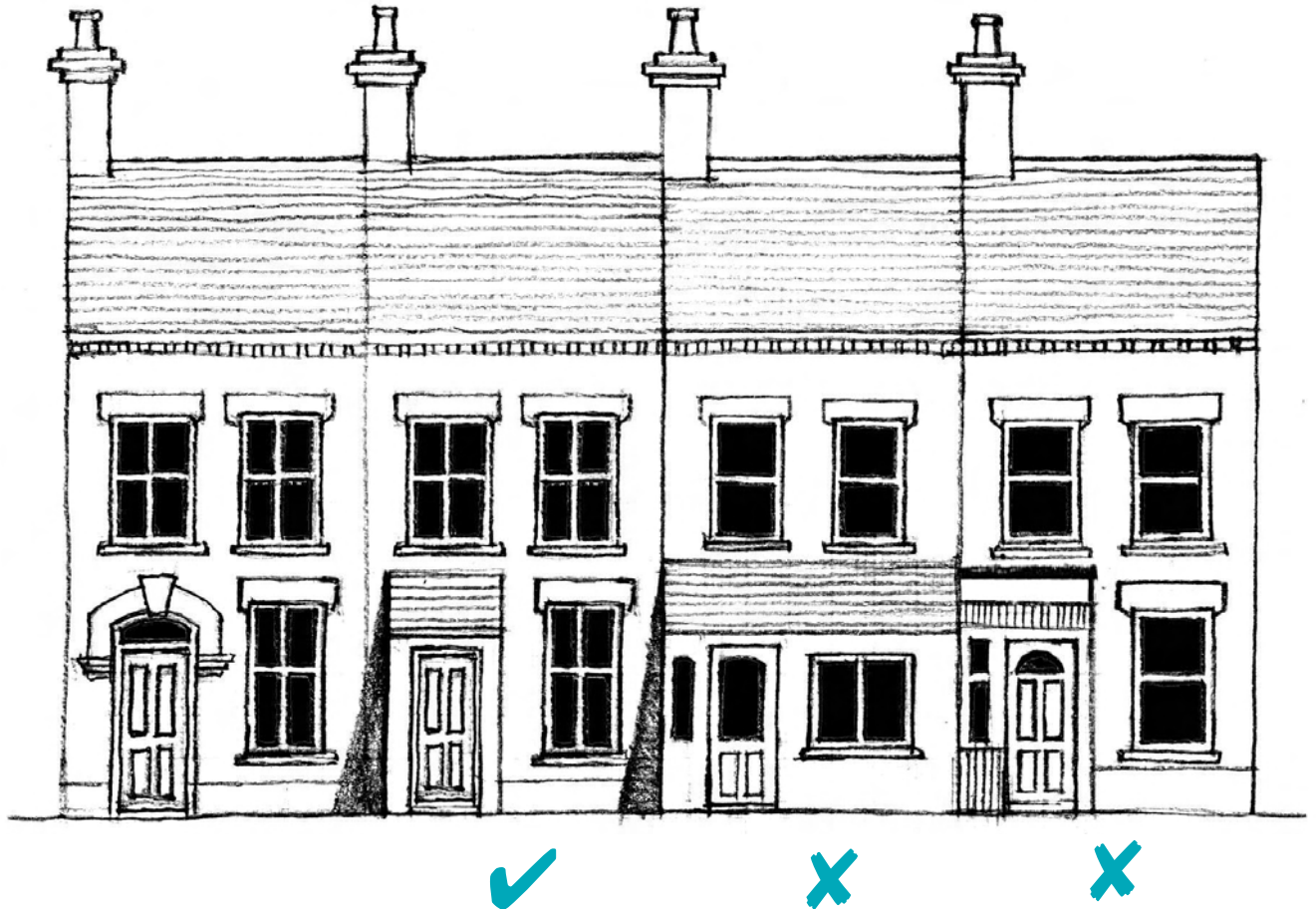
Acceptable porch extension to a terrace house 'fit in' with the existing appearance of the house.
