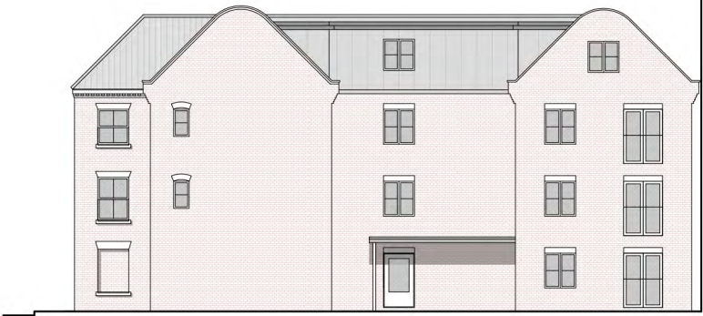
Proposed West Courtyard Elevation Grey standing seam cladding to rear dormers, lead grey single ply roof finish with PPC trims
