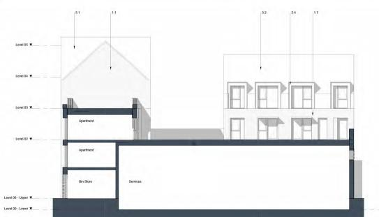
2 M - 05 - West Elevation Internal
