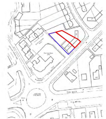
Site Location Plan (Site boundary - Red Ownership of adj. land - Blue) Scale 1:1250
