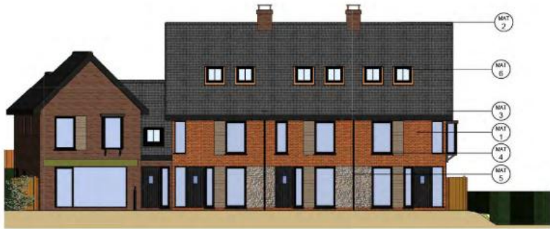
West Elevation - Front 1:100
