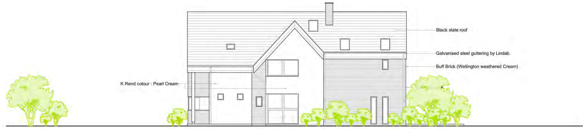
North West Elevation 1:100
