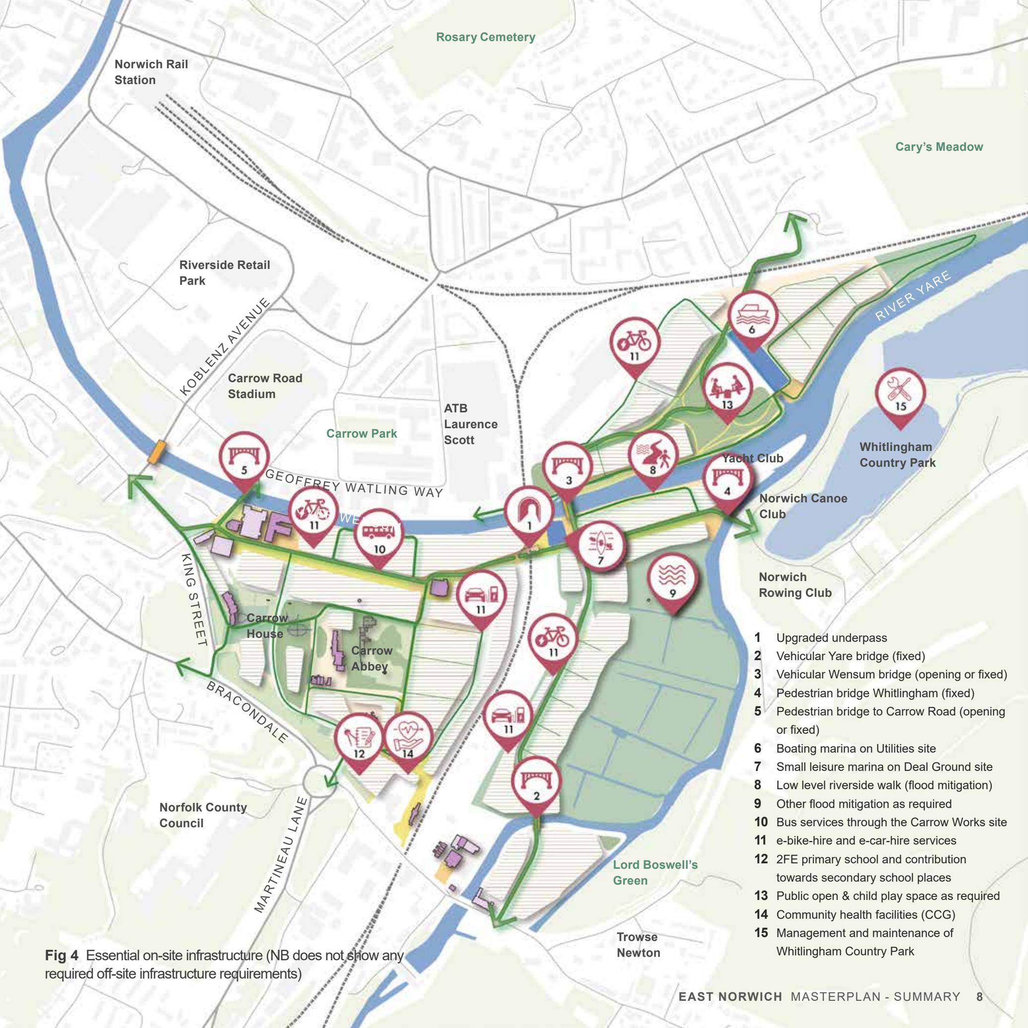
**Fig 4** Essential on-site infrastructure (NB does not show any required off-site infrastructure requirements)
