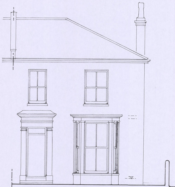
06.01 EAST FRONT ELEVATION, PROPOSED 1/50
