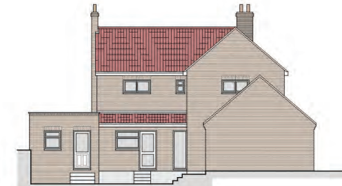
Existing Rear Elevation 1:100 @ A1
