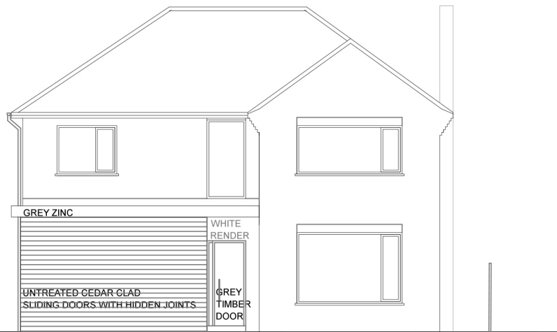
PROPOSED SOUTH ELEVATION - SCALE 1:100
