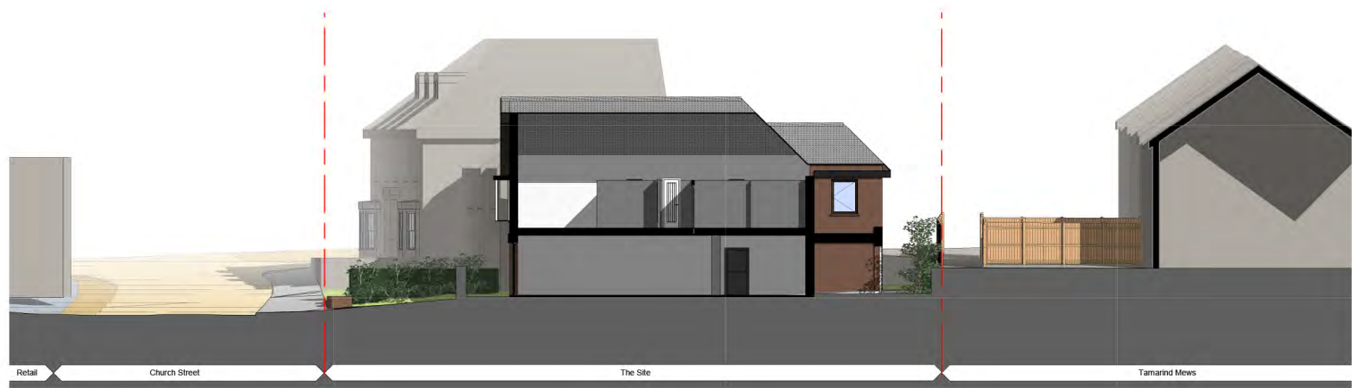
Short Section Through Commercial Unit
