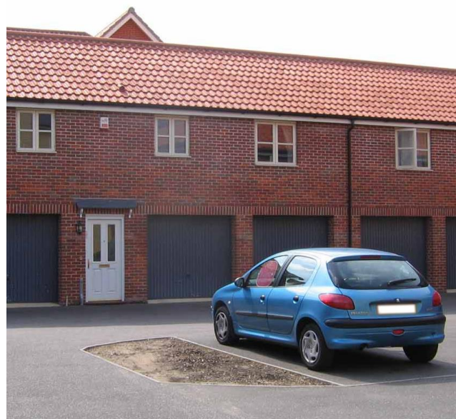
Failure of small isolated planting bed within parking area
