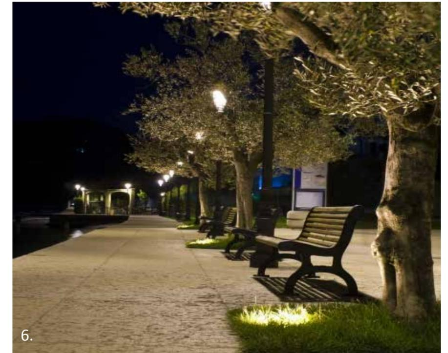
Images 4 & 5; use of shorter columns to illuminate environment below the tree canopies. Columns should respect the existing listed columns within the space and not dominate.
