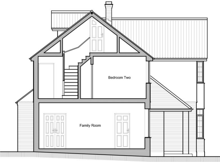
Proposed Indicative Section A-A
