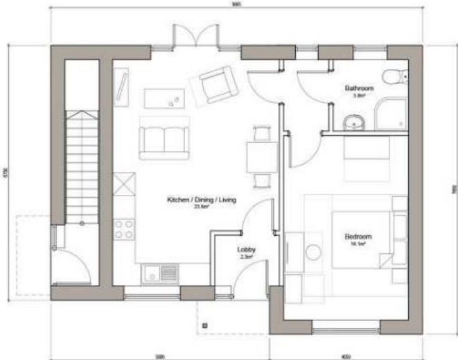
Ground Floor Plan Plot 1 1b2p Flat 50.00m² GIA (+5.48m² stairwell for upper floor flat)
