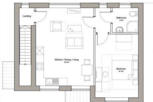
First Floor Plan Plot 2 1b2p Flat 55.04m² GIA (incl stairwell)
