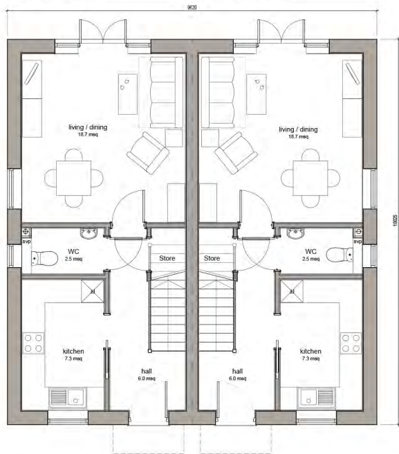
Plot 1 Ground Floor Plan 2b4p House 79m² GIA Plot 2 Ground Floor Plan 2b4p House 79m² GIA
