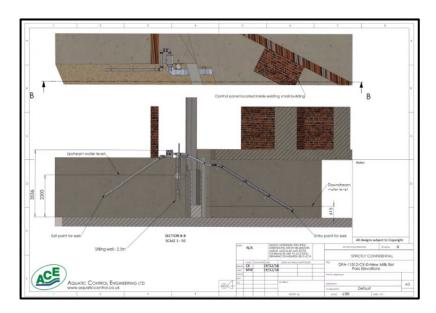
Figure 3: Elevation drawings showing the installed eel pass at New Mills (obtained from planning permission submission<sup>2</sup>)
