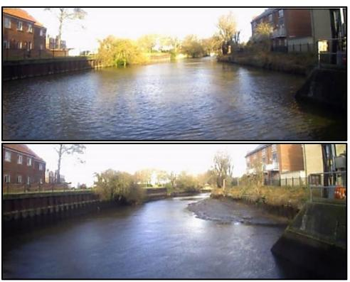
Figure 7: Photographs showing the effects of the New Mills draw down on water level before (top) and after with the exposed silt banks (bottom).
