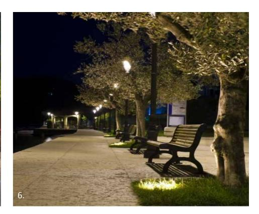
Image 6; up-lighting of trees could be used in combination with shorter columns.
