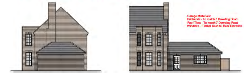
Proposed Garage Side Elevation 1:200 @ A1
